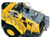
Serrated steps, wide catwalks and large handrails allow safe and easy access to the cab and to maintenance check points.
