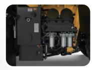
Filters and greasing points are centralized to make daily maintenance and servicing easier.
