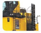
Serrated steps, wide catwalks and large handrails allow safe and easy access to the cab and to maintenance check points.
