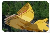
Additional strength has been added to the bucket bottom corners, side edges, and spill guard ends for increased durability.
