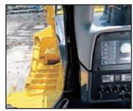
of the fuel tank allows the operator to have a clear view on the total width of the dozer back side, not only on the ripper point. This improves the ripper efficiency and safety level.
