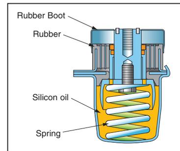
over adverse ground conditions. The cab damper spring isolates the cab from the machine body, suppressing vibrations and providing a quiet, comfortable operating environment.
