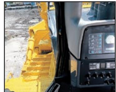
of the fuel tank allows the operator to have a clear view on the total width of the dozer back side, not only on the ripper point. This improves the ripper efficiency and safety level.
