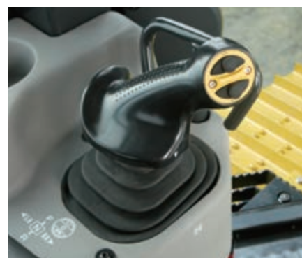
PCCS-Bedienhebel (Palm Command Control System)
