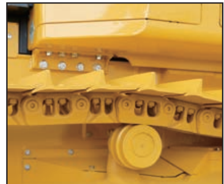
Komatsu Parallel Link Undercarriage System (PLUS)
