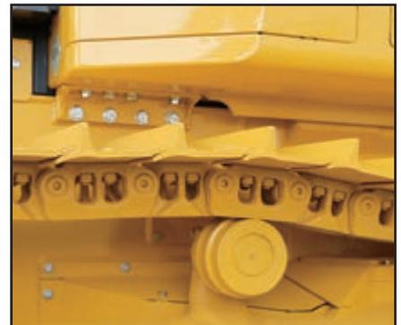
Komatsu Parallel Link Undercarriage System (PLUS)
