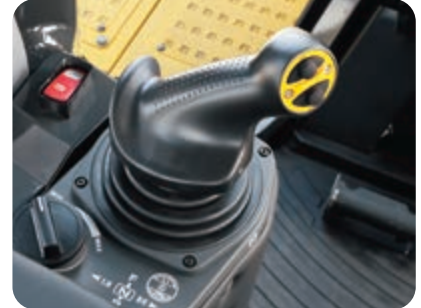
PCCS-Bedienhebel (Palm Command Control System)
