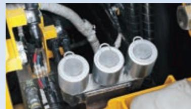
Canister-type breathers facilitate checking and cleaning
