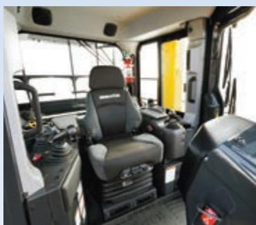
The seat is now fixed at a 12° angle to allow highest comfort for dozing and ripping
