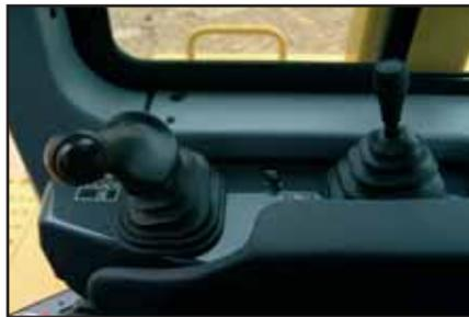
Blade and ripper control joystick
