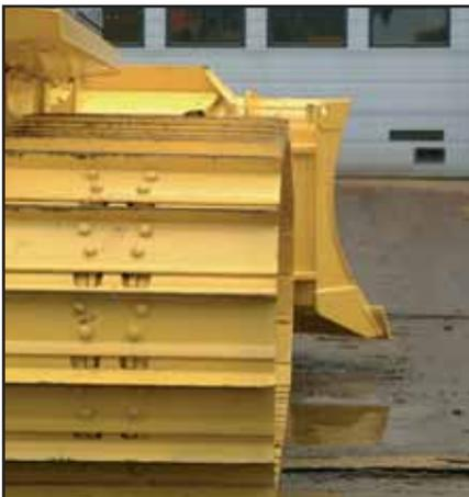
Unfolded blade (for operation)
