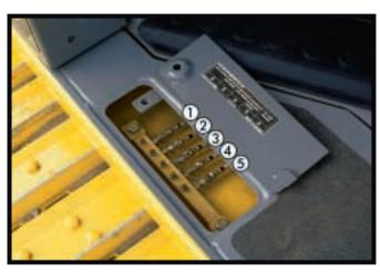
Centralized Oil Pressure Ports. The D61 offers the Komatsu exclusive centralized test ports on the right side of the chassis.
