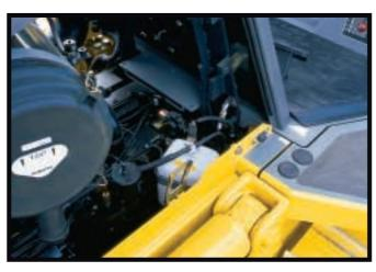
A radiator coolant reservoir makes it easier to check the coolant level and eliminates frequent refilling.
