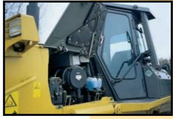
Gull-Wing Engine Side Covers with a gas-spring cylinder that opens widely, the engine and the auxilliary components can be checked easily.
