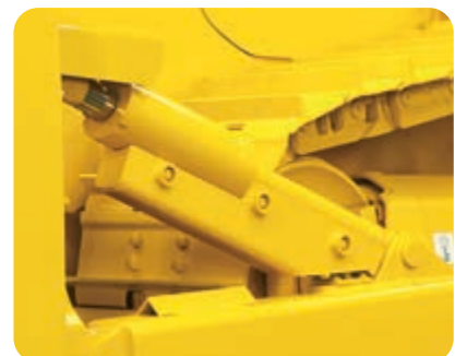
Hydraulic lines are embedded into the structures whenever possible
