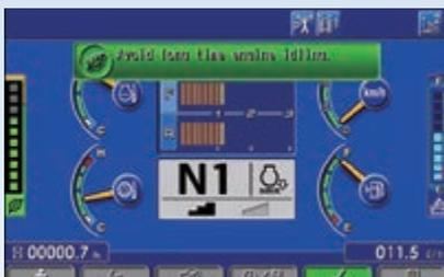
Eco gauge (left), Eco guidance tips and fuel consumption gauge (right) encourage efficient operation.
