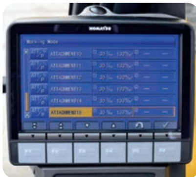
Komatsu Integrated Attachment Control (KIAC) for up to 15 tool presets for oil flow and pressure
