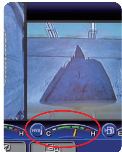
Hybrid system temperature gauge
