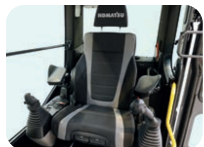
Optional premium seat with top quality cushioning, auto weight adjustment, lumbar support, climate control system, available with optional multi-position armrests and ergonomic control levers
