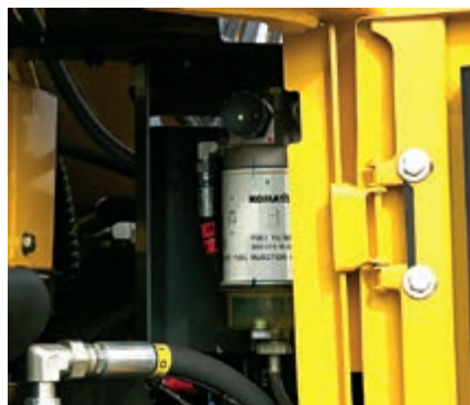
Fuel pre-filter with water separator
