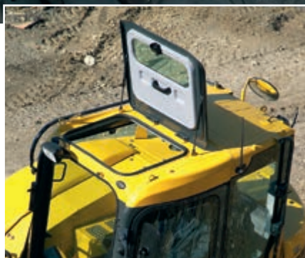
Opening skylight for overhead visibility
