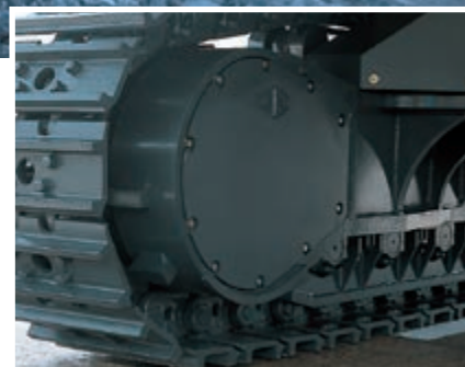
Sturdy travel motor guards and rock protectors
