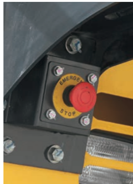
Three emergency engine stop switches are installed in the cab and around the machine, as standard.
