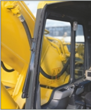
Visibility has been enhanced with additional window area by attaching the wiper to the cab frame.
