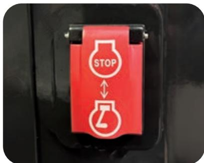
Secondary engine shutdown switch
