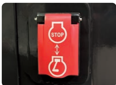
Secondary engine shutdown switch
