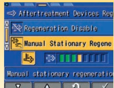
Aftertreatment device regeneration screen for the DPF
