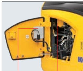
Washer tank Additional filter for breaker
