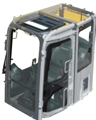
Optionally it can be fitted with an ISO 10262 Level 2 Operator Protective Guard (OPG) with openable front guard.
