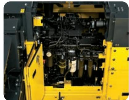
Centralised arrangement of filters
