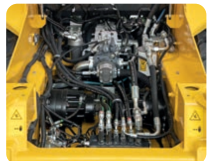
The tiltable cab can be raised in just a few minutes, providing easy access to the main valve and key hydraulic components
