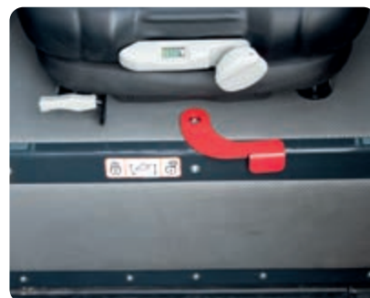
Work equipment safety lock lever
