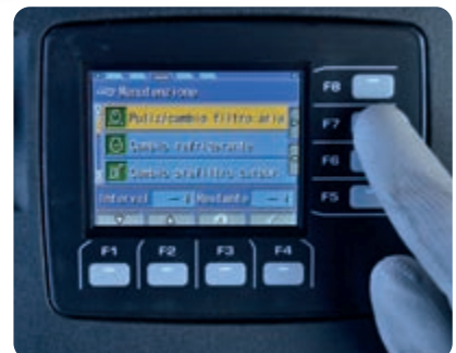
Basic maintenance screen on the 3.5" multi-colour monitor
