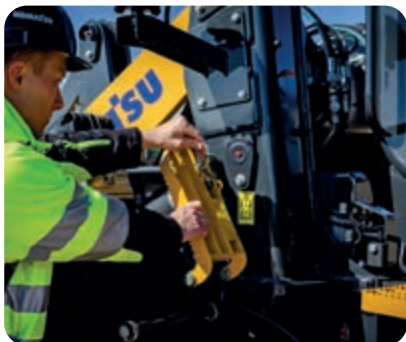
Front step for windshield cleaning
