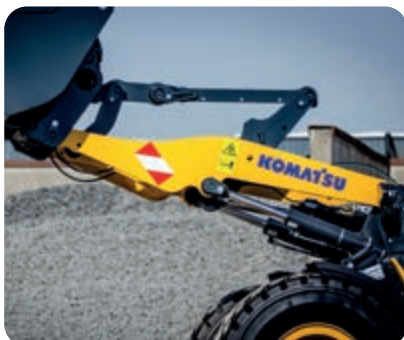
Tool linkage or Z-bar boom (option)
