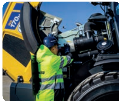
Ground level access to daily maintenance points
