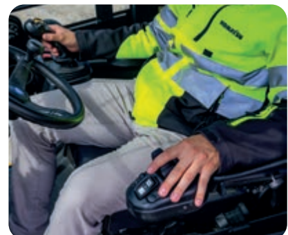
Integrated right-hand console moves with operator seat for outstanding operator comfort
