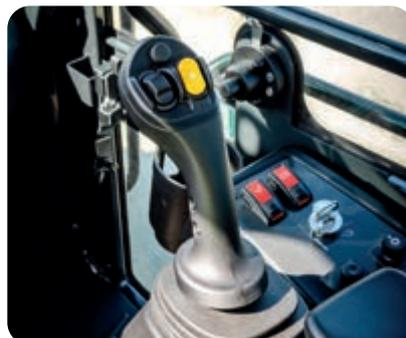
PPC multifunction lever with electronic control for 3rd hydraulic auxiliary circuit
