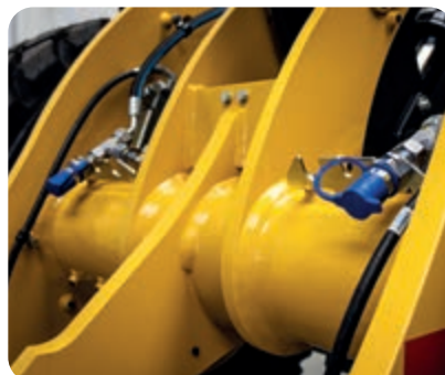
High flow for 3rd auxiliary circuit (160 l/min at 220 bar)
