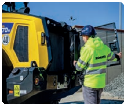
Wide core radiator with swing-out fan
