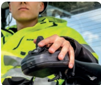
Komatsu Short-Lever Joystick Steering (K-SLS) (option)
