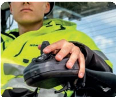
Komatsu Short-Lever Joystick Steering (K-SLS) (option)
