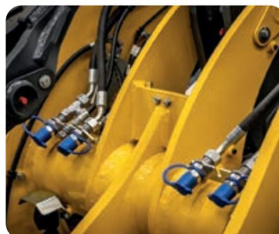
High flow for 3rd auxiliary circuit
