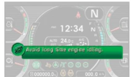
Eco guidance supports energy saving in real time (e.g. avoid long time engine idling)
