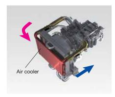
Air-to-air charge air cooling system
