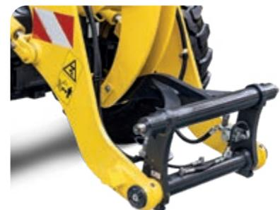
Electrically actuated quick-coupler for fast and easy change of attachments
