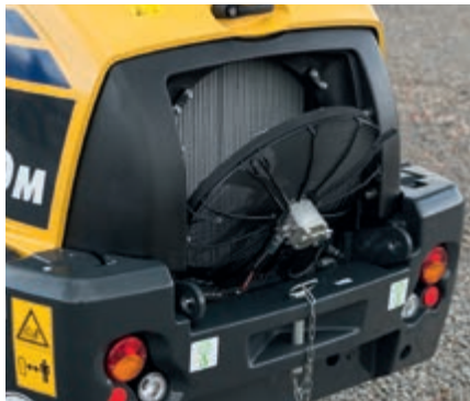
Tiltable radiator fan for convenient cleaning access
