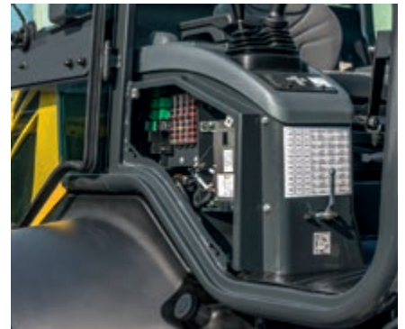
Side cover for quick maintenance access
