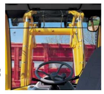
As an option, it is available the LSS (Load Stabiliser System) acting on loader lifting cylinders.
