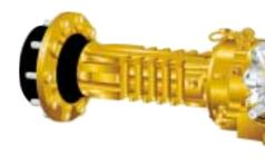
Maximum operating safety is also guaranteed by the excellent braking system. Oil immersed multidisc brakes can be independently operated by either of the two foot pedals. Pressing both pedals together automatically activate four wheel drive.
