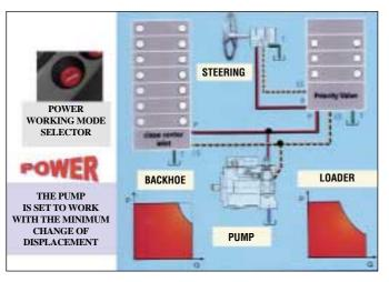
The system consists of a single variable flow hydraulic pump and an "intelligent" hydraulic circuit that allows the machine to adapt instantaneously to the specific operation being carried out. The CLSS (Close Load Sensing System) type circuit, together with the variable flow pump, means that only the amount of oil strictly necessary for ensuring high operating
