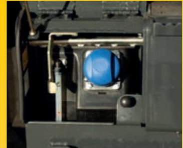
AdBlue®, fuel and hydraulic oil tank are easily accessible on the machine side and refilled by ground level, ensuring a fatigue less operation
