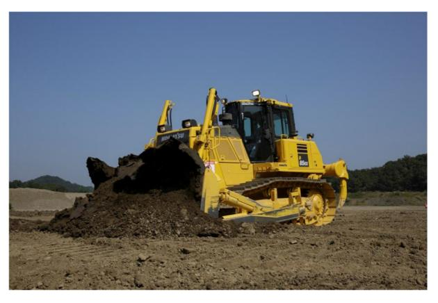
*Vilvoorde, March 2015* — Komatsu Europe International N.V introduces the D85EX/PX-18 crawler dozer. With operating weights ranging between 26.800 kg and 30.190 kg (depending on machine configuration), the D85EX/PX-18 is powered by a Komatsu SAA6D125E-7 engine that is EU Stage IV emissions certified and with a net 197 kW (264 HP).
