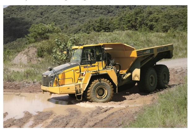
Vilvoorde, January 2014 — Komatsu Europe International N.V. announces the introduction of the Komatsu HM400-5 Articulated Dump Truck (ADT) to the EU market. Presented at CONEXPO-CON/AGG 2014 in Las Vegas, the HM400-5 is powered by a Komatsu SAA6D140E-7 engine that is EU Stage IV emissions certified and with a net 353 kW (480 HP).
