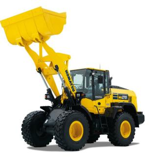
*Vilvoorde, December 2016* — Komatsu Europe presents the new WA270-8 wheel loader, an all-around utility performer for almost any worksite, with an attachment-friendly quick coupler, an EU Stage IV engine and up to 3 % lower fuel consumption.
