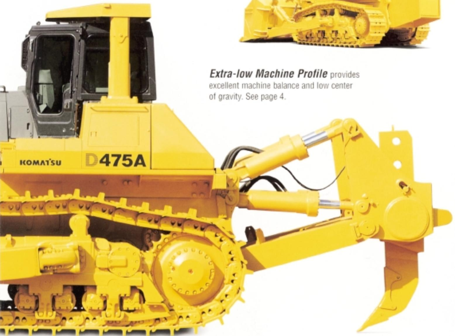
**Resilient Equalized Undercarriage (REU)** improves traction, component durability, and operator comfort. See page 6.
